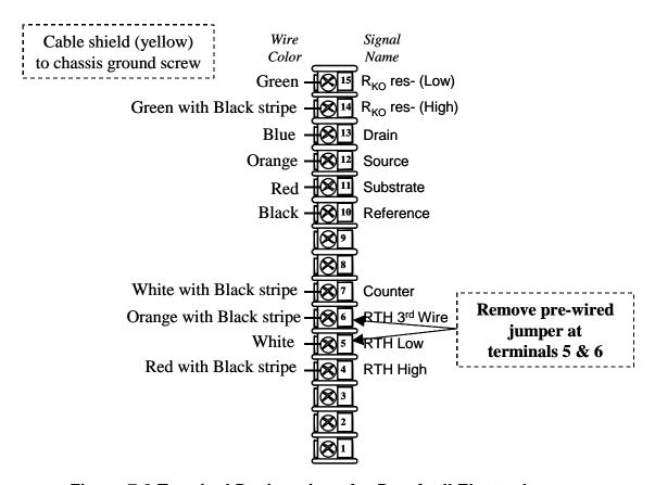
Figure 7-3 Terminal Designations for Durafet II Electrode
